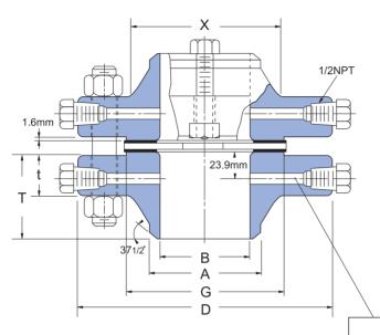
$\frac{1}{4}^{''}$  Drill for Sizes  $2\frac{1}{2}^{''}$  and Under  $\frac{3}{8}^{''}$  Drill for Sizes  $3^{''}$
