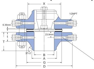
$\frac{1}{4}^{''}$  Drill for Sizes  $2\frac{1}{2}^{''}$  and Under  $\frac{3}{8}^{''}$  Drill for Sizes  $3^{''}$
